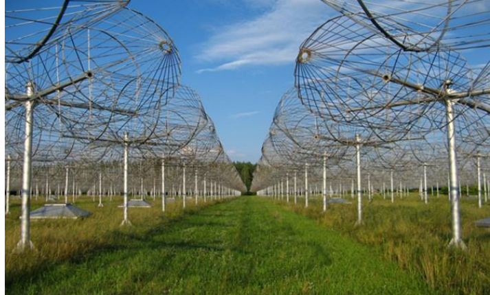
Figure 16: URAN-2 radio telescope of NASU, Ukraine, observes radio emission generated in the solar corona at heliocentric distances 2-3 solar radii.
