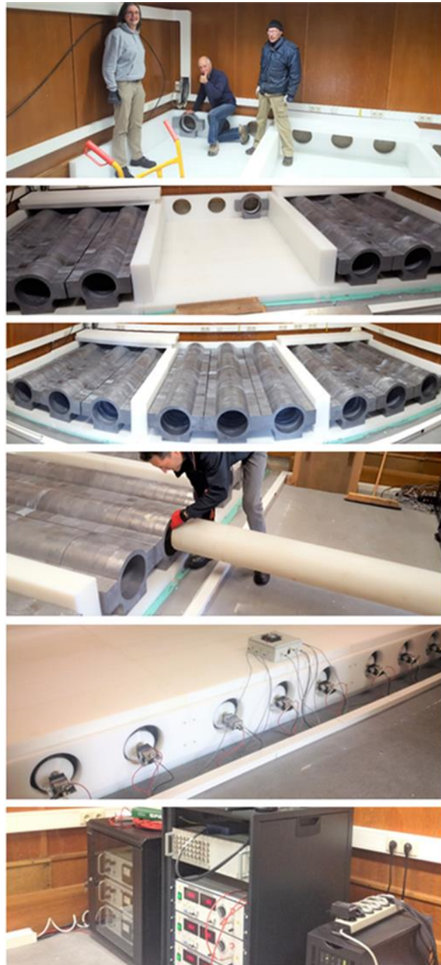
Figure 27: Construction of the new neutron monitor at Dourbes - from design to assembly, testing and start of the continuous monitoring of cosmic rays intensities.
